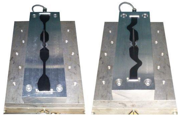
Fig. 10 Production of test sample by injection molding
