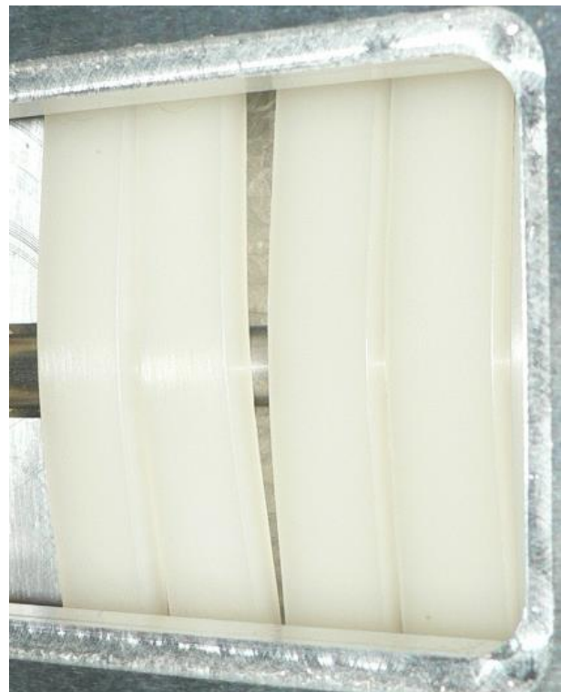
Fig. 12 Irradiated PA11 specimens placed in the reference environment
