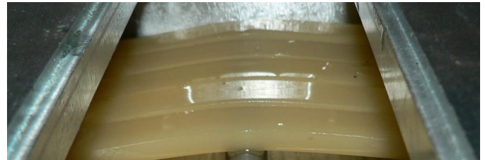
Fig. 16 Non-irradiated PA12 specimens placed in the brake fluid environment after 168 hours
