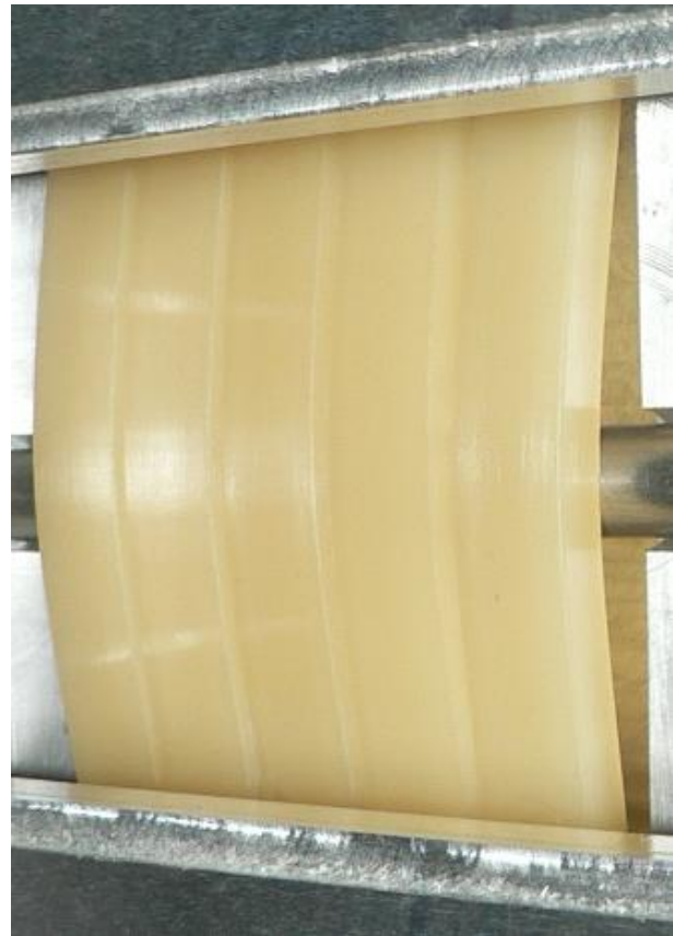
Fig. 10 Non-irradiated PA12 specimens placed in the reference environment
