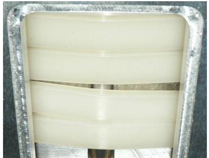
Fig. 15 Irradiated PA12 specimens placed in the reference environment after 168 hours
