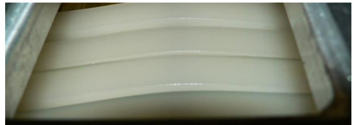
Fig. 17 Irradiated PA12 specimens placed in the brake fluid environment after 168 hours
