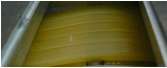
Fig. 12 Non-irradiated PA12 specimens placed in the brake fluid environment
