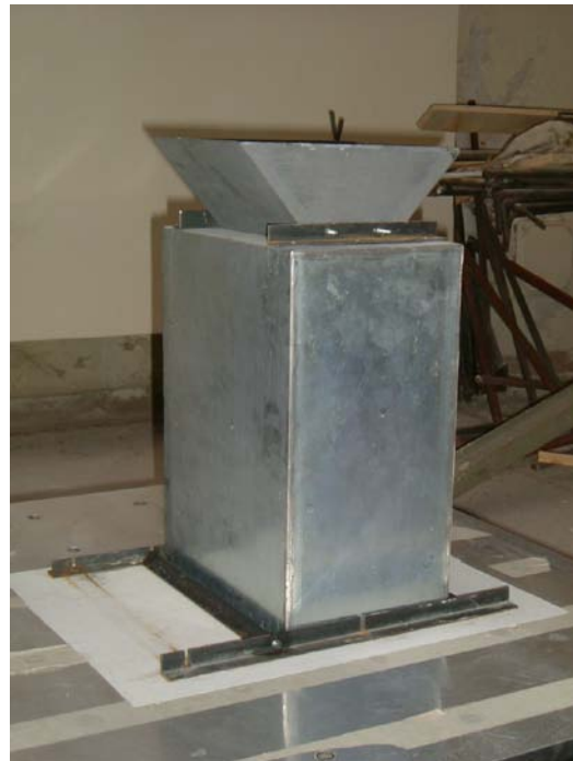
Fig.2– Sample of tests executed in Naples on aluminum blocks equipped with TLD.
