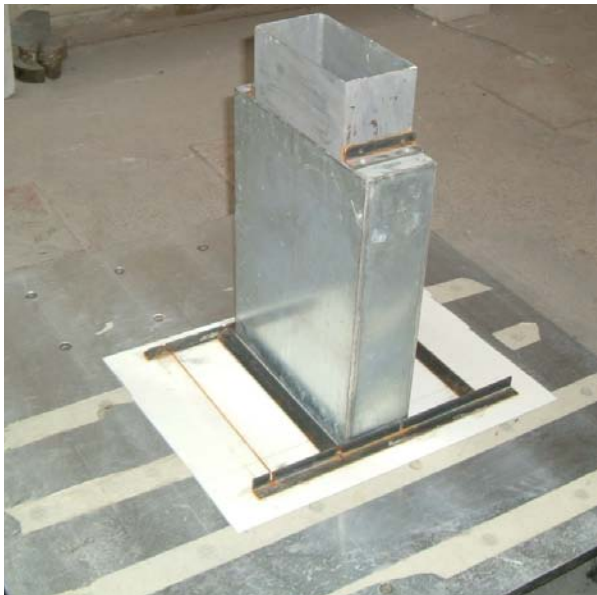
Fig.3– Sample of testing in Naples on aluminum blocks equipped with TLD.
