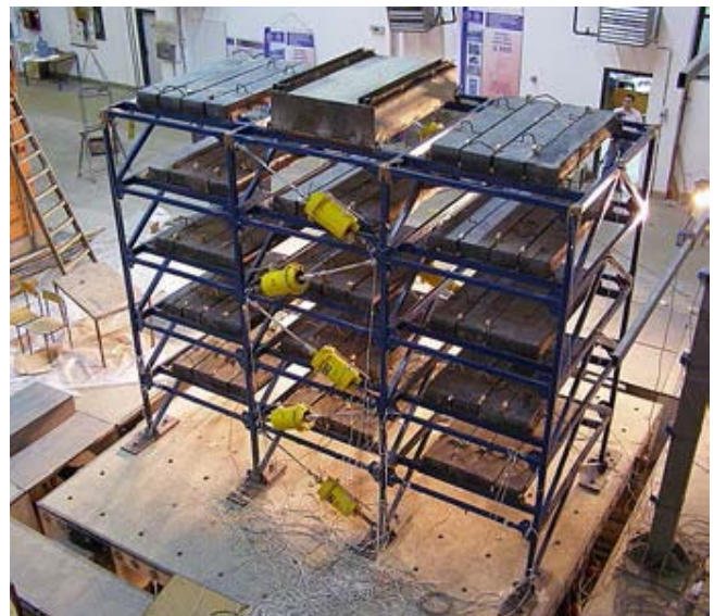
Fig.6 – Geometry of the steel frame tested to IZIIS.
