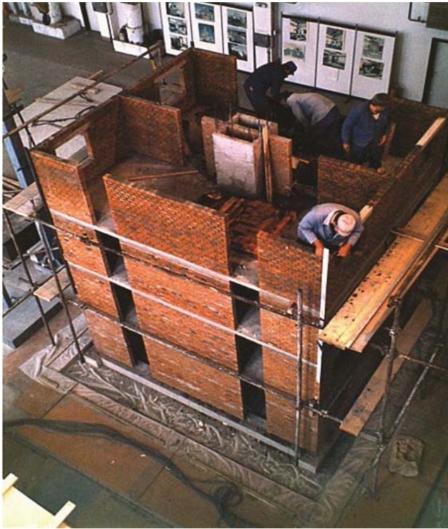
Fig.8 – Some testing on a masonry multi-plane structure in IZIIS.
