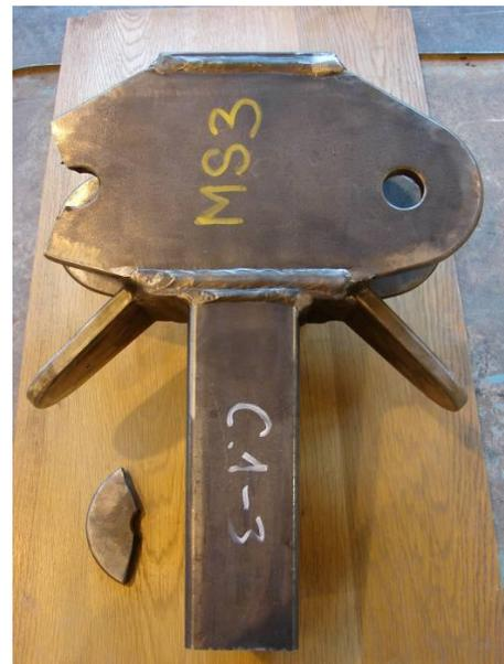
Fig. 17 Illustration of typical fatigue failure – cracks around holes for pins: joint middle part
