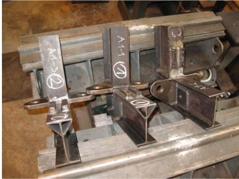
Fig. 7 Illustration of produced assembly joints of short footbridge main girder lower chord: specimens including transverse frame
