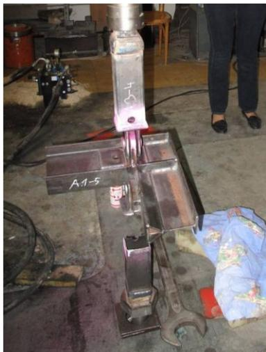
Fig. 13 Illustration of typical fatigue failure – cracks near welds on end parts of lower chords: specimen including transverse frame
