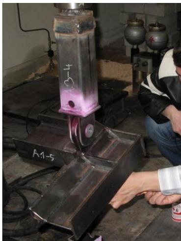
Fig. 9 Illustration of tests of short footbridge main girder lower chord: specimen including transverse frame
