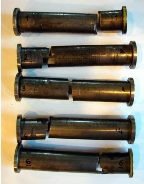
Fig. 15 Illustration of typical fatigue failure – failed pins
