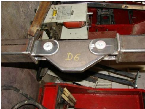
Fig. 8 Illustration of produced assembly joints of short footbridge main girder upper chord: specimen not-including transverse frame
