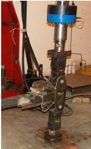
Fig. 12 Illustration of tests of long footbridge main girder lower chord
