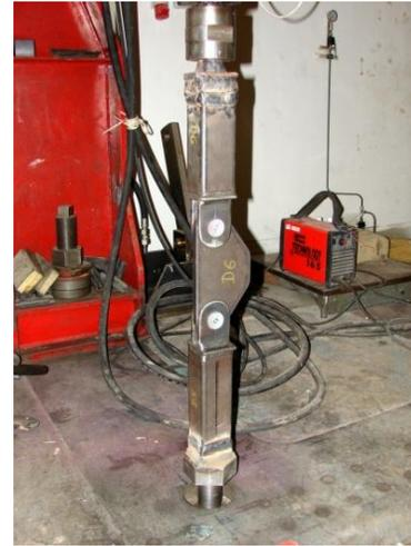
Fig. 10 Illustration of tests of short footbridge main girder lower chord: specimen not-including transverse frame
