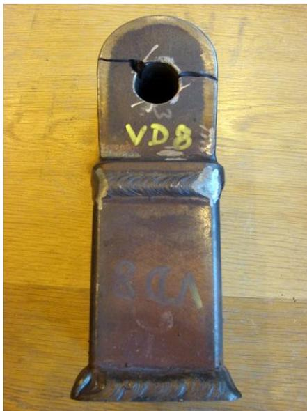
Fig. 16 Illustration of typical fatigue failure – cracks around holes for pins: chord end part
