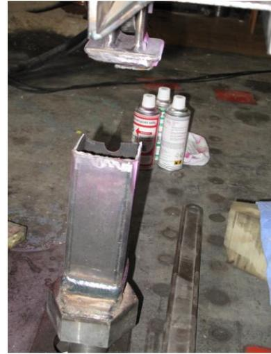
Fig. 14 Illustration of typical fatigue failure – cracks near welds on end parts of lower chords: specimen not-including transverse frame
