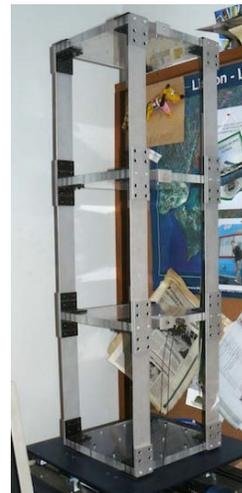
Figure 3: Metallic scaled frame at the shaking table.
