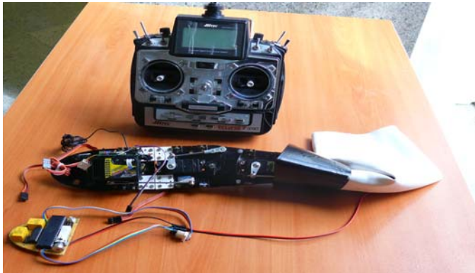
Fig. 9 servomotors and controller
