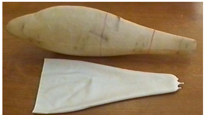
Fig. 8 the outer body of the robot fish and its waterproof skin
