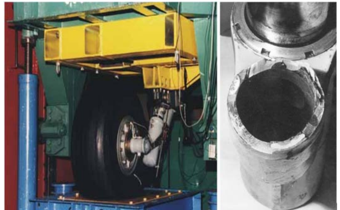
Fig. 1 view of the drop stand and the failure of the top landing gear's leg
