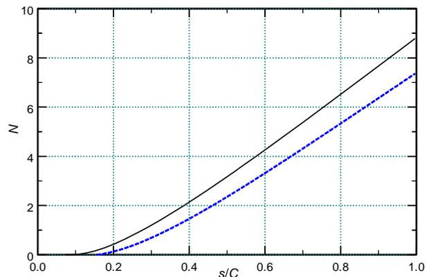
**Fig.13:** Growth curves (N-factors) of stationary ( $\omega = 0$ ) cross-flow instability modes, computed for conditions of measurements [10]: local self-similar solution (solid line) and full boundary layer solution (dashed line); spanwise wave length  $\lambda = 2\pi/\beta = 7$  mm.
