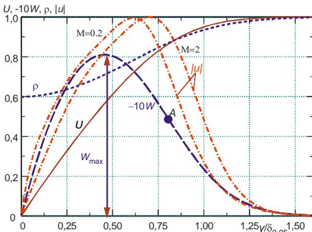
**Fig.2:** Mean flow parameters for  $M_e = 2$  and fluctuations of the longitudinal velocity of the steady ( $\omega = 0$ ) model of instability of the transverse flow for  $\beta = 1.3$  and  $R = 5000$ .
