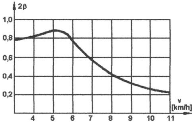
Figure 4 The variation of 2\beta according to speed, for the collision of two cars equipped with 75 mm bumpers
