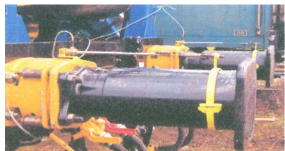
Figure 23 D 3 - Coupling system displacement car A/car B
