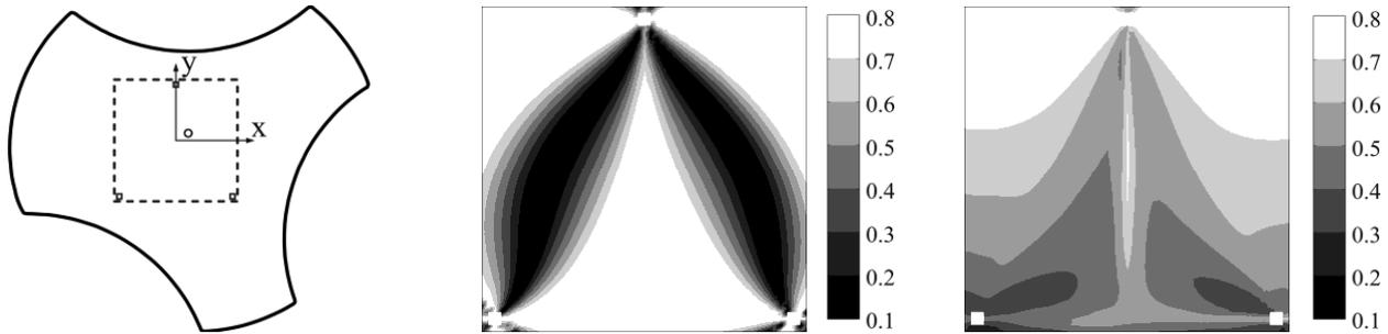
Fig. 3 Correlation index maps of isotropic (centre) and unidirectional (right) laminates.
