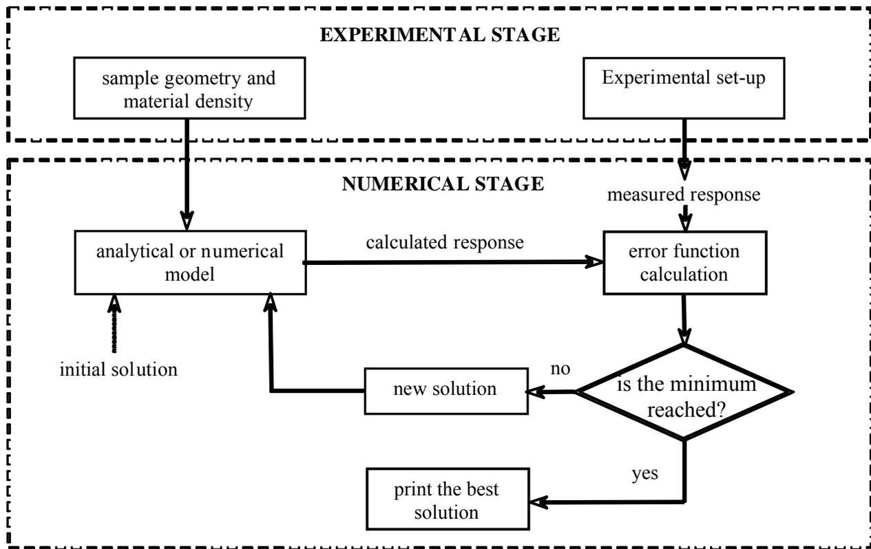
Fig. 2 Schema of a procedure for the elastic characterization of materials.
