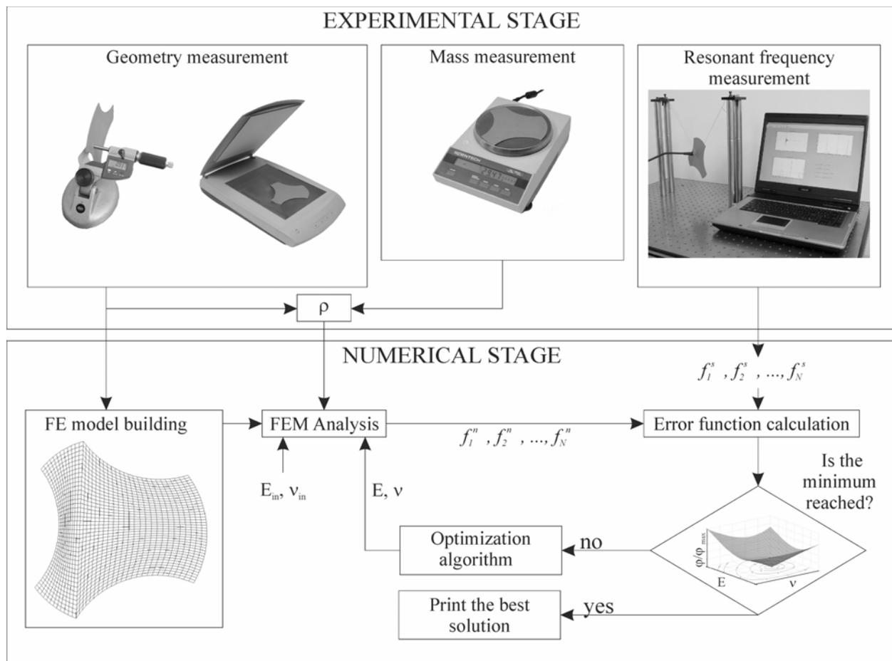
Fig. 6 Elastic identification via dynamic test [20].
