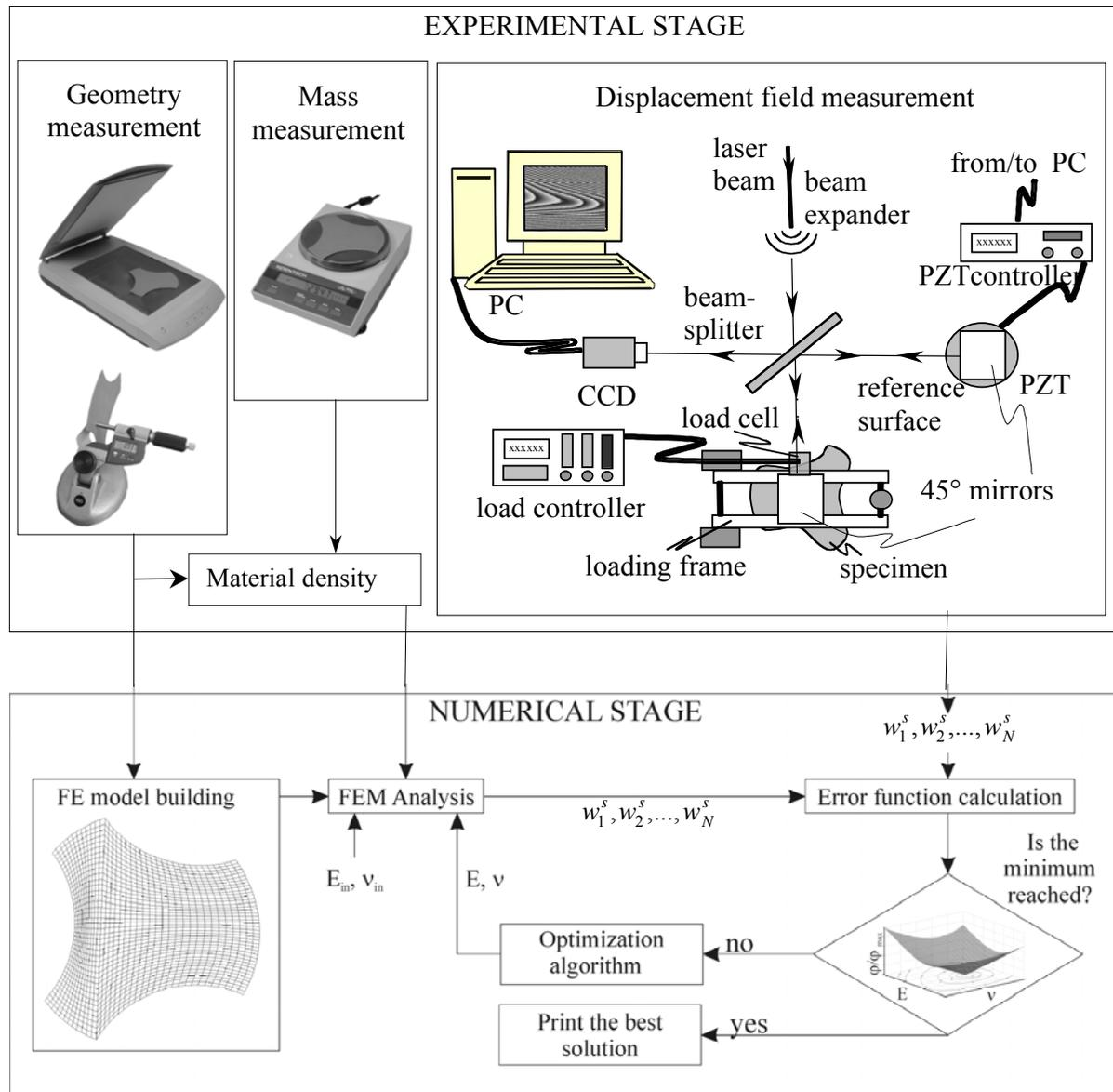
Fig. 4 Elastic identification via static test.
