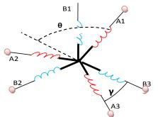
Fig.01.shows the winding of the DSIM
