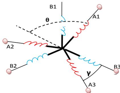
Fig.01.shows the winding of the DSIM
