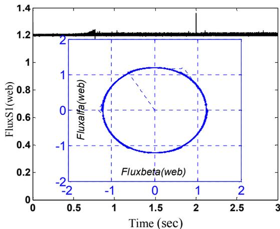
Fig.5.4.show the Direct and quadratic stator flux of ANN DTC
