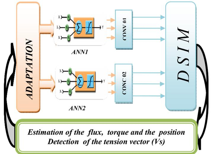
Fig.2.1. Block diagram of the Artificial Neural Network direct control of torque Application on the DSIM
