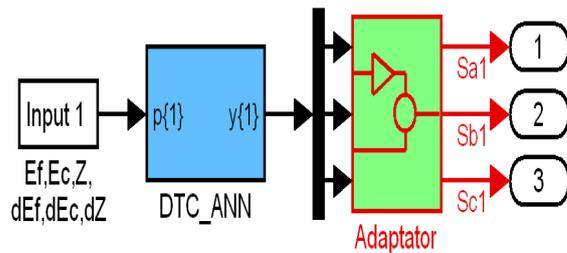
Fig.4.3. Model simulink of ANN used in DTC of DSIM
