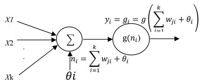
Fig.3.2. Single node in an artificial neural network.
