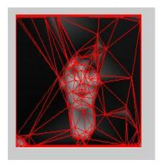
Refinement the mesh SOM maps with finite elements
