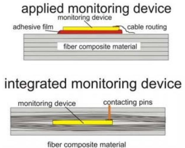
Fig. 6: Applied (up) and integrated (down) device comparison
