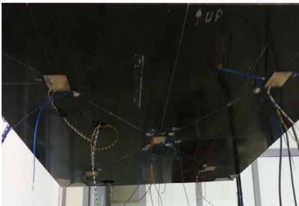
Fig. 1: Piezoceramic patches bonded on the panel
