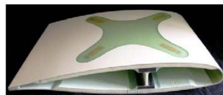
Fig. 7: Embedded PZT fiber transducer
