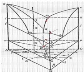
Figure 1 Space model of ternary phase diagram
