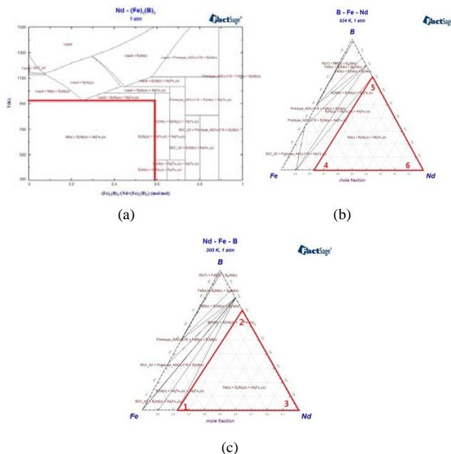
Figure 2 (a) Vertical section; (b) Isothermal section at temperature 924(K); (c) Isothermal section at temperature 300(K)
