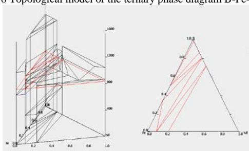
Figure 7 Isothermal section diagram at temperature 924(K)
