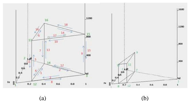
Figure 5 (a) Phase region  $\text{Nd(s)}+\text{B5Nd2(s)}+\text{Nd5Fe17(s)}$ ; (b) Phase region  $\text{B4Nd(s)}+\text{Nd2Fe17(s)}+\text{Nd5Fe17(s)}$
