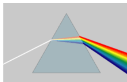
Figure.1 Prism which separates light into monotonic colors
