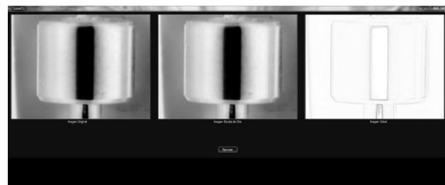
Fig.6. Micro piston image after Sobel operator application
