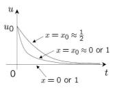
Fig. 14. The temperature against time curve obtained by Hancork, valid for  $t \geq 1/\pi^2$ , comparable to the solution in Fig. 13.
