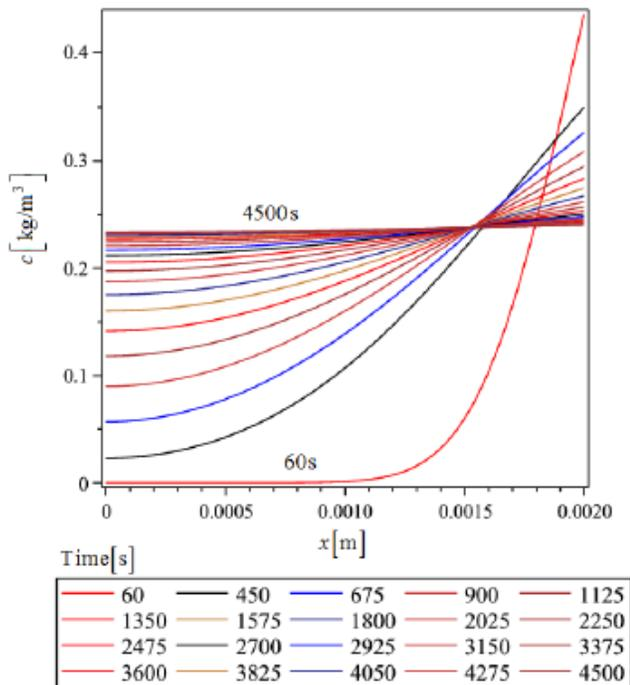
Fig. 2 Concentration fields of alkali in specific time of dechromatization
