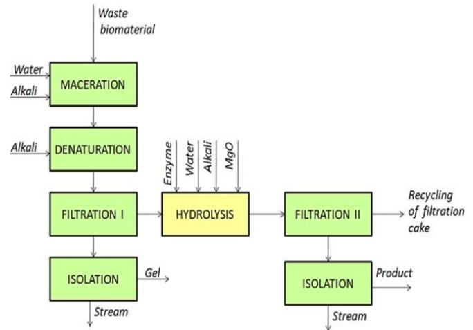
Fig. 3 Enzymatic hydrolysis - manufacturing scheme
