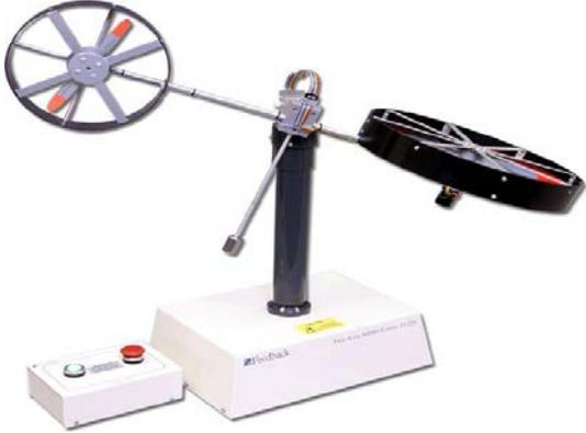
Fig. 1 Twin Rotor MIMO System
