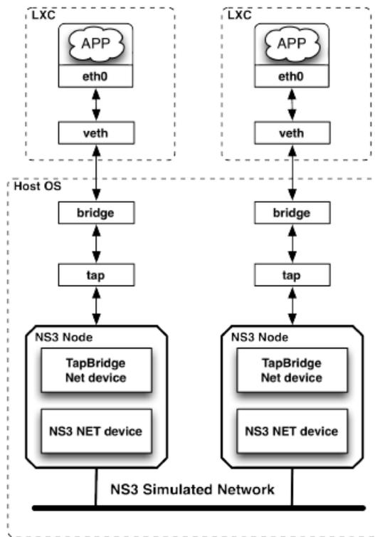
Fig. 3: LXC connectivity via veth and tap devices
