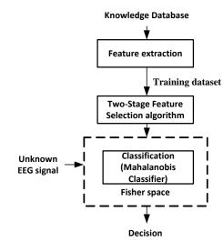
Fig.1 Block diagram of automatic diagnosis process
