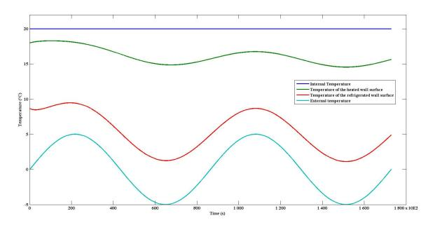
Fig. 6. Simulation results: internal temperature  $\theta_{w10}$ , external temperature  $\theta_{w20}$ , temperature of the heated wall surface  $\theta_{w1}$ , temperature of the refrigerated wall surface  $\theta_{w2}$  with input conditions parameters  $c, \rho, d_w$ .
