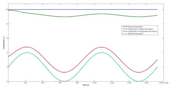
Fig. 5. Simulation results: internal temperature  $\theta_{w10}$ , external temperature  $\theta_{w20}$ , temperature of the heated wall surface  $\theta_{w1}$ , temperature of the refrigerated wall surface  $\theta_{w2}$  with input conditions parameters  $c, \rho, d_w$ .
