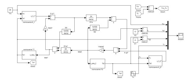
Fig. 4. Simulation model heat transfer dynamic through the wall.
