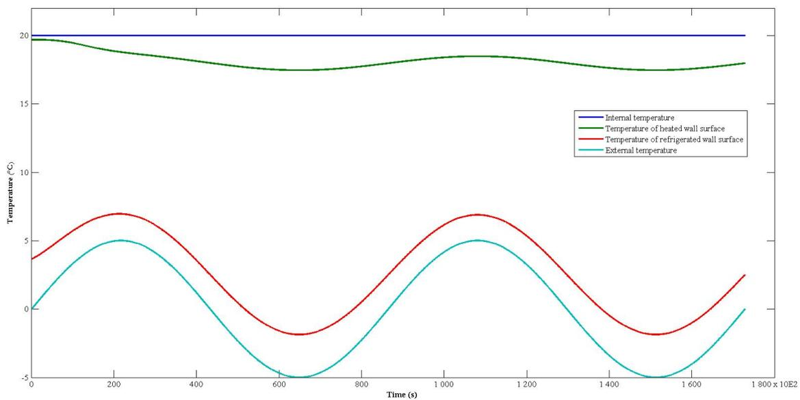
Fig. 5. Simulation results: internal temperature  $\theta_{w10}$ , external temperature  $\theta_{w20}$ , temperature of the heated wall surface  $\theta_{w1}$ , temperature of the refrigerated wall surface  $\theta_{w2}$  with input conditions parameters  $c, \rho, d_w$ .
