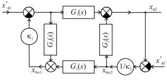
Fig. 3. Block diagram with  $x_{\phi_1}^*$ ,  $x_{\phi_2}^*$
