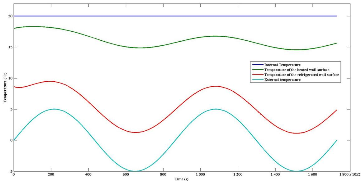
Fig. 6. Simulation results: internal temperature  $\theta_{w10}$ , external temperature  $\theta_{w20}$ , temperature of the heated wall surface  $\theta_{w1}$ , temperature of the refrigerated wall surface  $\theta_{w2}$  with input conditions parameters  $c, \rho, d_w$ .
