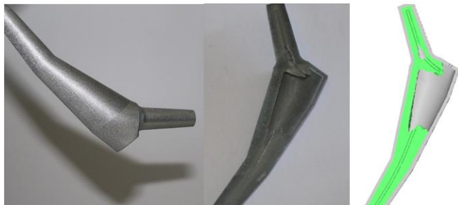
Figure 6 : optimization example for additive manufacturing
