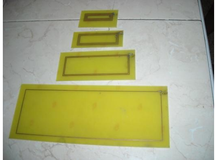
Fig.8: Antenna loops made
