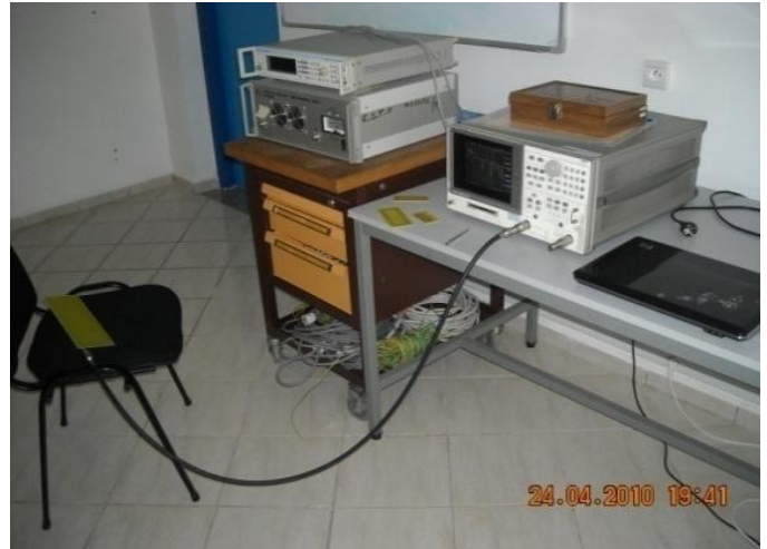
Fig.9: Measurement of the reflection coefficient of the antenna using a vector network analyzer.
