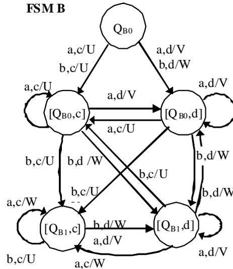
Fig. 8 back transformation of the FSM B'
