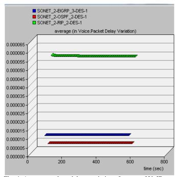
Fig. 4. Average packets delays variations for case of VoIP applications.
