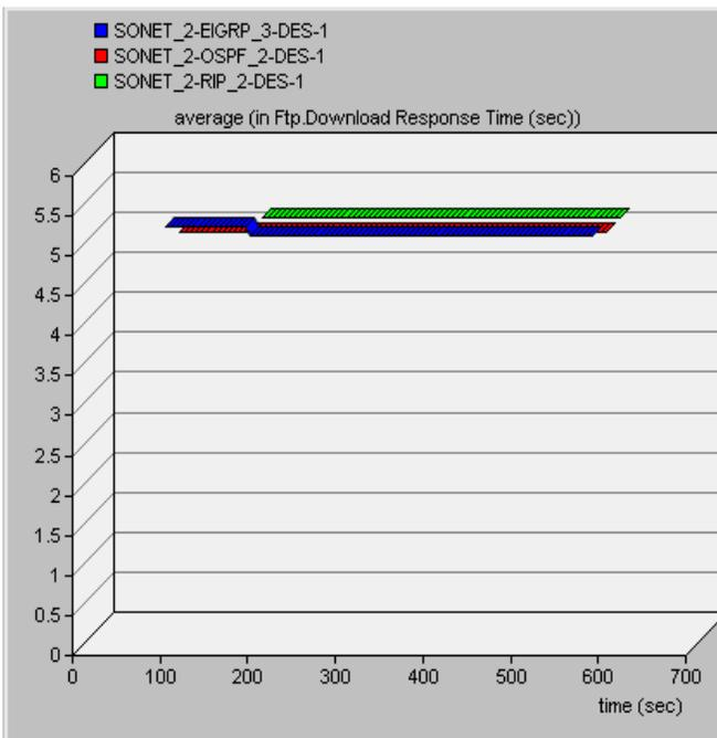
Fig. 8. Average response time for downloading FTP files.
