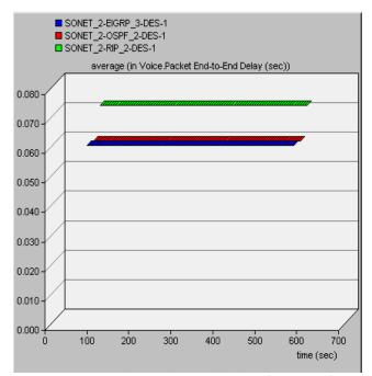
Fig. 5. Average packets end-to-end delays for case of VoIP communication.
