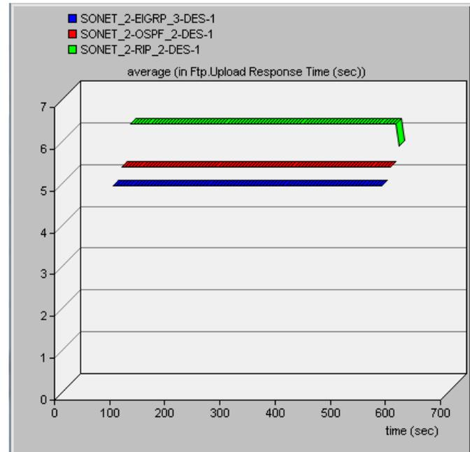
Fig. 9. Average response time for uploading FTP files.
