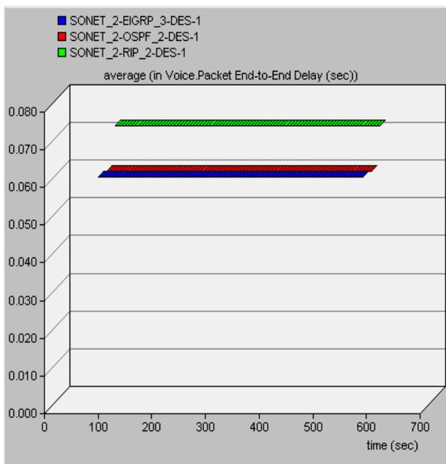
Fig. 5. Average packets end-to-end delays for case of VoIP communication.
