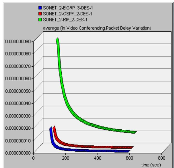
Fig.2. Average packets delays variations for case of video applications.
