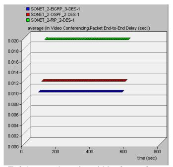
Fig.3. Average packets end-to-end delays for case of Video applications.
