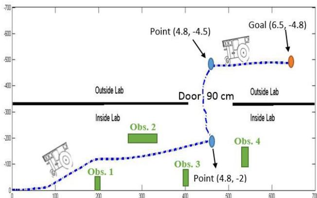
Figure 18: Robot experimentation in unknown environment with static and dynamic obstacles
