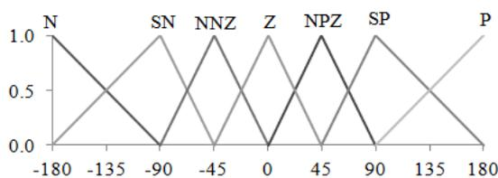
Figure 4: Membership functions for the angle error.
