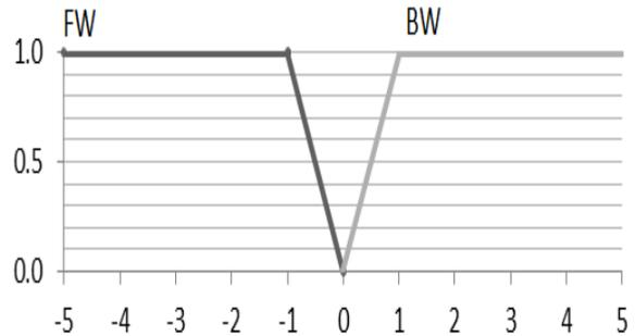
Figure 15: Membership functions of the Left & Right Velocity of RSM.
