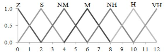
Figure 5: Membership functions of LV and RV Near Medium, M: Medium, NH: Near High, H: High, and VH: Very High. The influence rules of the LV and RV are defined in Table 1.
