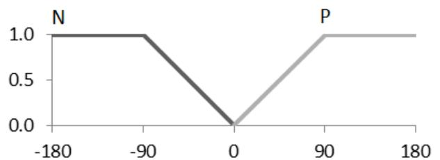
Figure 16: Membership functions for the error in angle of the RSM.
