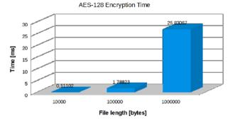
Fig. 20 AES-128 Encryption time
