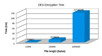
Fig. 17 DES Encryption time
