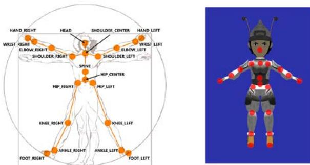
Fig. 5. Kinect Skeleton Joint and Implementation Character Bone
