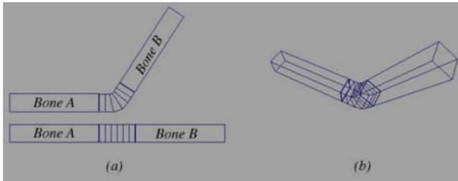
Fig. 8. Skinning Mesh & Vertex Blending
