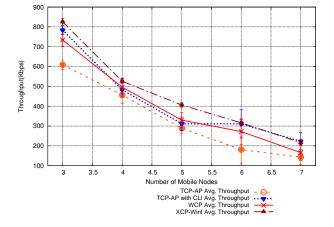
Figure 7. 16 Mesh Nodes - Variable Number of Mobile Nodes, *TCP-AP with CLI* Throughput.
