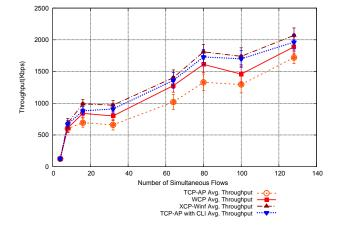
Figure 10. Ad-Hoc Scenario, TCP-AP with CLI Throughput.
