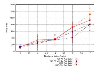
Figure 8. 16 Mesh Nodes - Variable Number of Mobile Nodes, *TCP-AP with CLI* Delay.
