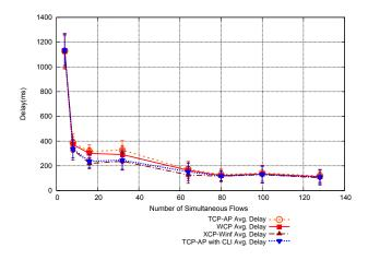
Figure 11. Ad-Hoc Scenario, TCP-AP with CLI Delay.
