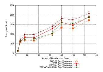
Figure 4. Ad-Hoc Scenario, TCP-AP with rt-Winf Throughput.
