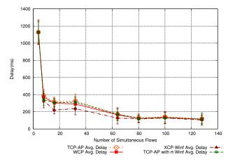
Figure 5. Ad-Hoc Scenario, TCP-AP with rt-Winf Delay.
