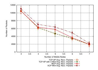
Figure 3. 16 Mesh Nodes - Variable Number of Mobile Nodes, *TCP-AP with rt-Winf Received Packets*.
