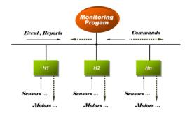
Fig. 1 The dataflow of the housing monitoring system
