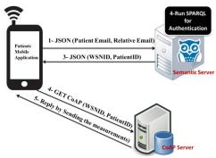
Figure 8-Authentication Process for Relative's mobile app.
