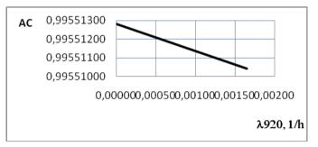
Fig 6. Graph of dependence of AC of SBC and the rate of transition to a state of Brute-force attacks -  $\lambda$ 920
