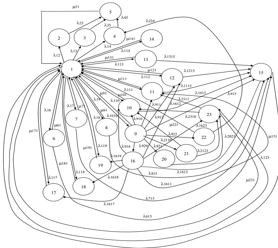
Fig. 2. Markov's graph of system SBC states
