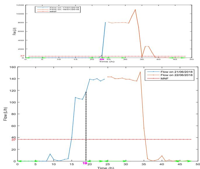
Fig. 8. Detecting a water leak by MNF.
