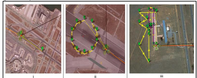
FIGURE 2 – Automated missions planned for quadcopter (i- Single waypoint; ii- Circular waypoint; iii- Random waypoint)
