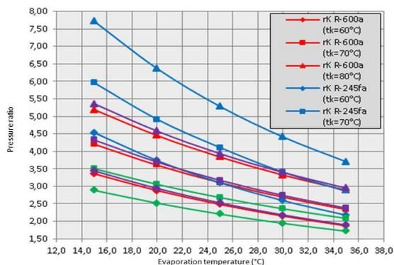
Fig. 11: Pressure proportion of the single phase heating pump
