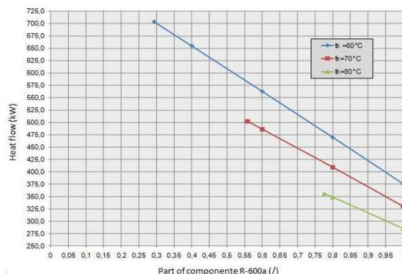
Fig. 6: Heating flow of the cooking part of the heating pump depending on the share
