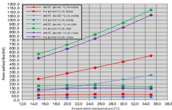
Fig. 7: Single phase heating pump at condensation temperature  $t_k=60^\circ\text{C}$
