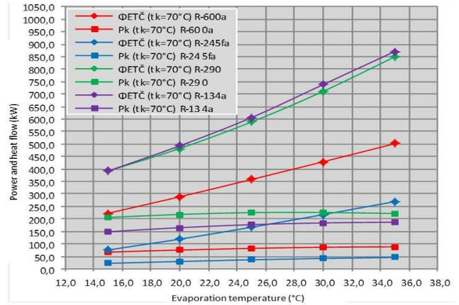
Fig. 8: Single phase heating pump at condensation temperature  $t_k=70^\circ\text{C}$
