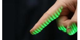
Fig 3. Flashscan's fingerprinting uses stripes of light to capture a 3D image with no touching
