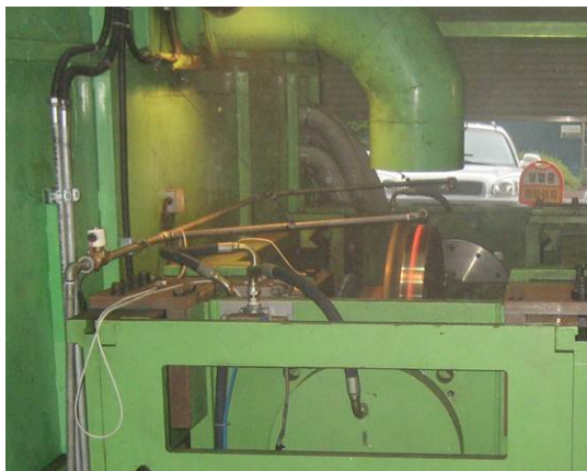
Fig.4 the shape of braking test and thermal band observed on the wheel when it is on braking
