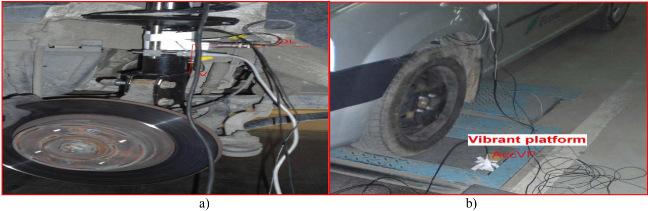
Fig. 3: Detail of: a) front suspension and positioning measurement transducers; b) the location of the platform side of the wheel vibratory equipped with transducers measure.
