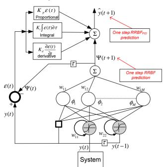
**Fig. 6.** The RRBF<sub>PID</sub> structure for time series prediction
