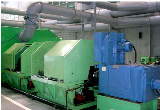
Fig. 2 brake performance dynamometer for high speed train
