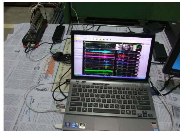
Fig. 7 measurement system for the brake experiment (DAQ)
