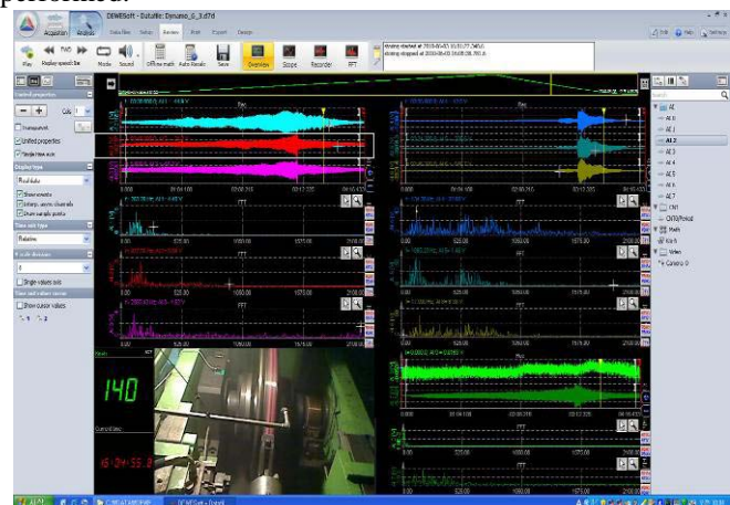
Fig. 10 DAQ screen for the analyzing the vibration
