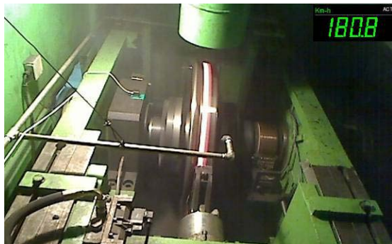
Fig.3 Tread braking test at 180 [km/h]
