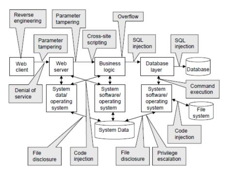
Fig. 2 Points of Vulnerability for a Web-application [3]
