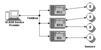
Figure 2 Common SCADA Installation utilizing Remote Terminals (PLC/DCS, Sensors) and Master Station connected using a fieldbus.
