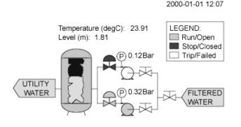
Figure 1. An Example of a SCADA Human Machine Interface
