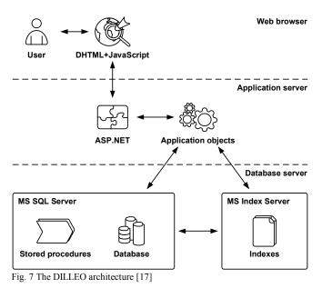
This is typical architecture of many contemporary information systems which produces tight coupled relations between application objects (components). Flexibility of such system is very low; it is very complicated and relatively expensive to customize certain parts and behavior of the software.
