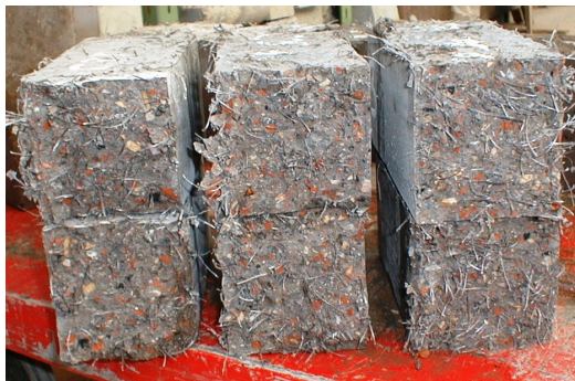
Fig. 7 Specimens with recycled masonry aggregate and synthetic fibres
