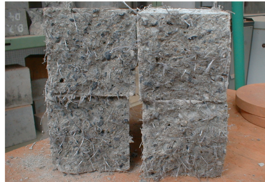
Fig. 8 Specimens with recycled concrete aggregate and synthetic fibres
