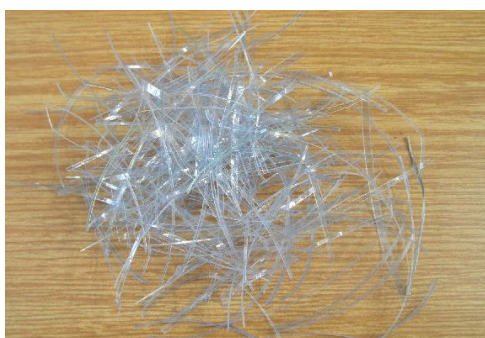
Fig. 10 Tested fibres from PET-bottles
