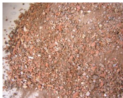
Fig. 4 Masonry rubble (fraction 0/32 mm) tested in experimental program
