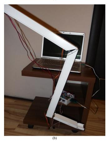
Fig.11 The virtual model (a) and the simple prosthesis (b) under the position tracking test
