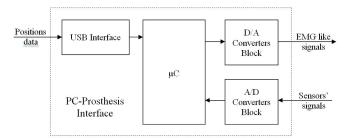
Fig.7 PC-Prosthesis interface block diagram
