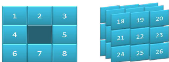
Figure 4-2: In 2D, each cell has 8 adjacent cells. In 3D, each cell has 26 adjacent cells. [26]
