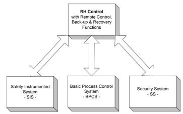
Fig 4 Functional Architecture incorporating Risk and hazard control
