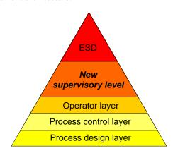
Fig. 1. Layers of protection
