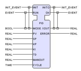
Fig. 7. The PID composite function block
