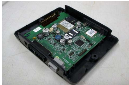
Fig. 7 picture of Telematic Control Unit considered in the case study (source: author)
