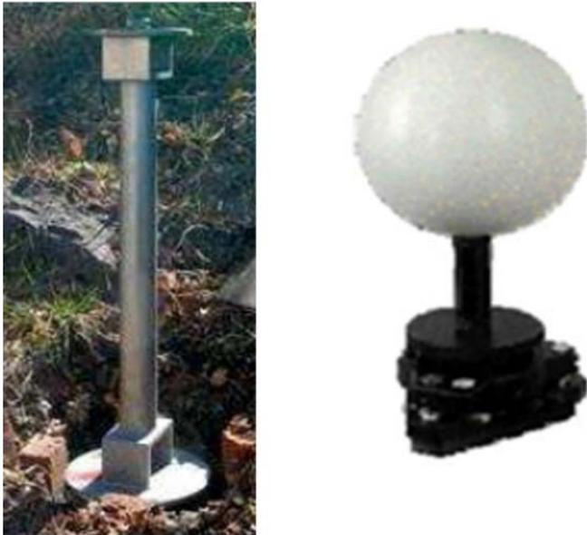
Fig. 12 spherical target in polystyrene 12 cm
